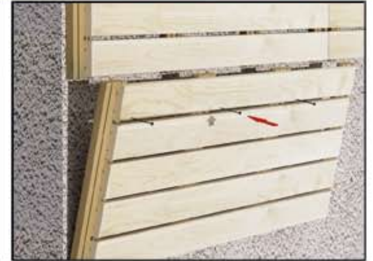
3-) Karkastan vidalı, gizli montajlı sistem Hidden installation system from carcass screwed
